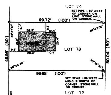
NOTE: CHAIN LINK FENCE ENCROACHES ON SOUTH LINE 0.6' NORTH OF SOUTHWEST CORNER AND 0.3' NORTH OF SOUTHEAST CORNER.
